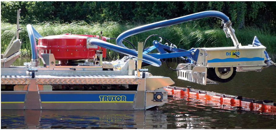
The Doro skimmer is equipped with a bracket where the suction tubing (Sala roll pump) is placed.
