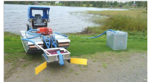
The Doro skimmer is equipped with a bracket where the suction tubing (Sala roll pump) is placed.
